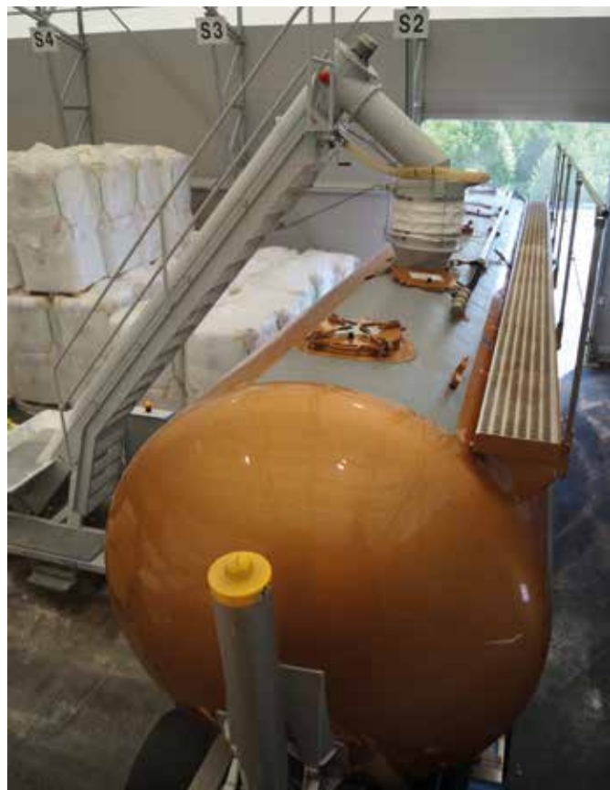
The company's own bulk terminal in Finland debags packed materials to bulk
